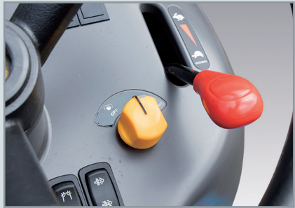
Independent PTO switch Turn the independent PTO on or off with a simple switch.
