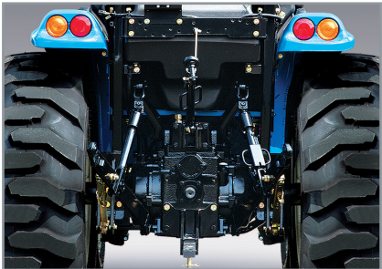
3-point hitch Category 1 with a hitch lift capacity of 2,910 lbs allows usage of wide variety of implements.
