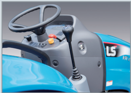
Fender mounted joystick for front end loader Easily accessible for maximum comfort and convenience.
